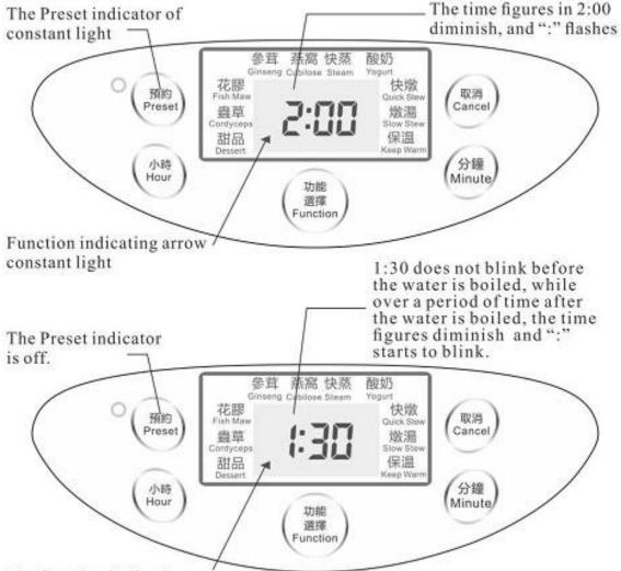
The function indicating arrow blinks before the water is boiled and it constant light after the water is boiled.
